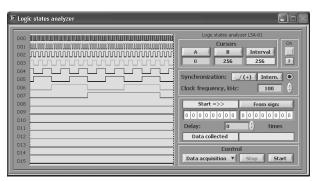
Fig. 6. Front panel of the logic state analyzer.
