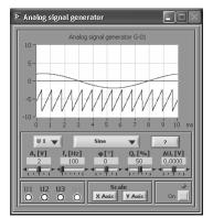
Fig. 1. Front panel of the arbitrage waveform generator.
