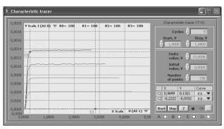
Fig. 5. Front panel of the two-terminal networks and four-terminal networks volt-ampere characteristic analyzer.
