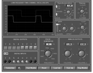
Fig. 10. The front panel of "Microcontrollers and signal processors" test bench
