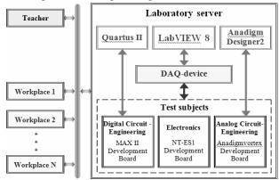
Fig. 10. Structure of universal laboratory "Electronics and Circuit-Engineering".
