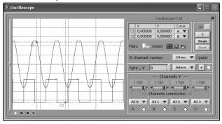
Fig. 2. Front panel of the 4-channel oscilloscope
