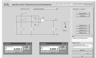
Fig. 8. Front panel of experimental software module for analog circuitengineering on the student workplace
